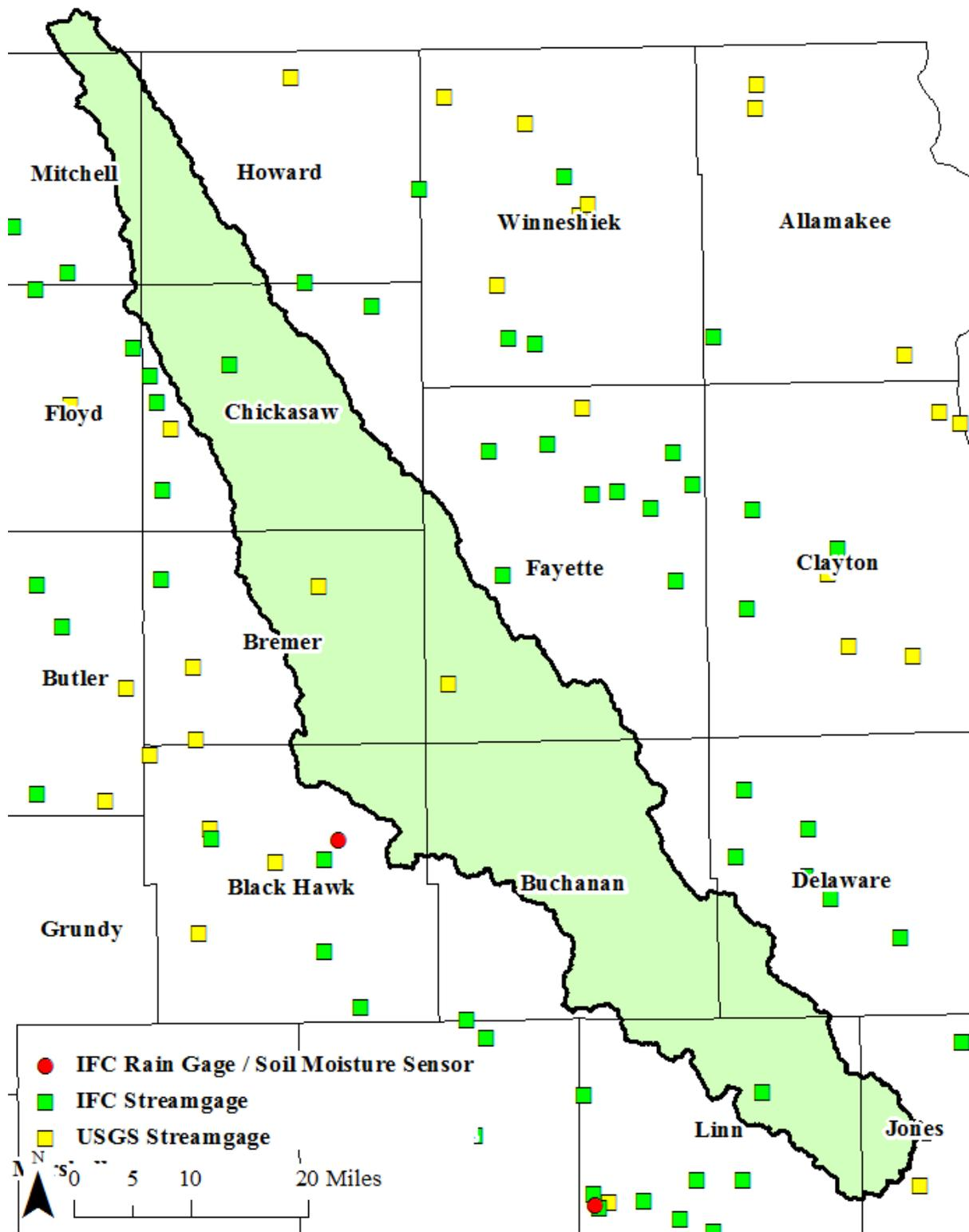
Figure 2.11. Hydrologic and meteorologic instrumentation in the Upper Wapsipinicon Watershed. Stage/discharge gages are shown in yellow or green while precipitation and soil moisture gages are shown in red.
