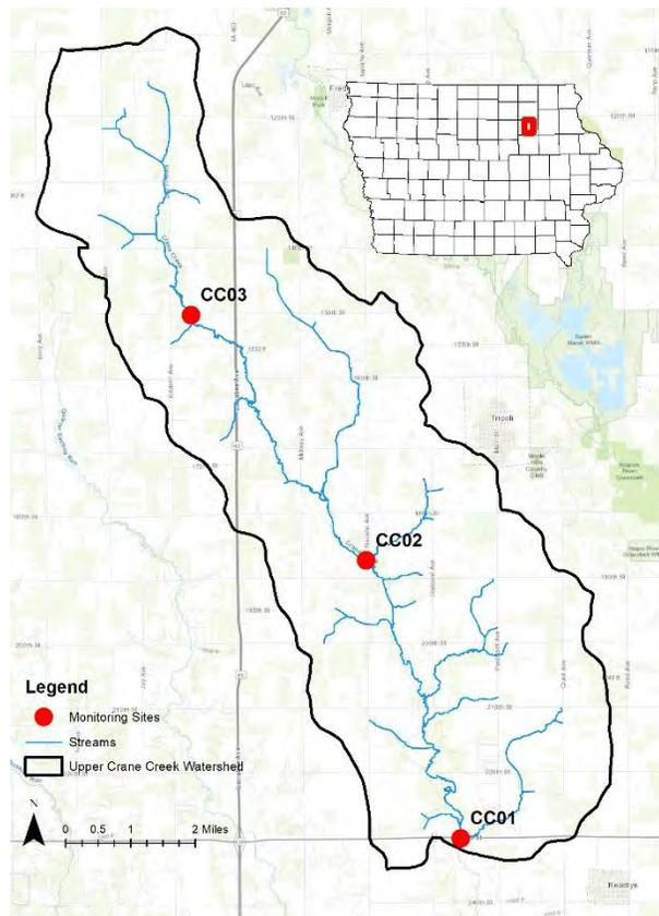
Figure 7.1.1. Recommended locations for collection of stream water samples in the Upper Crane Creek Watershed.
