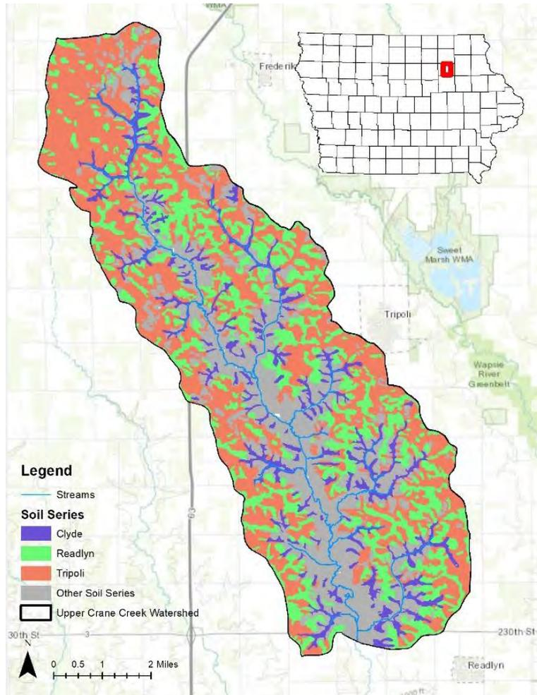
Figure 2.5.1. Upper Crane Creek Watershed soil map derived from SSURGO data.
