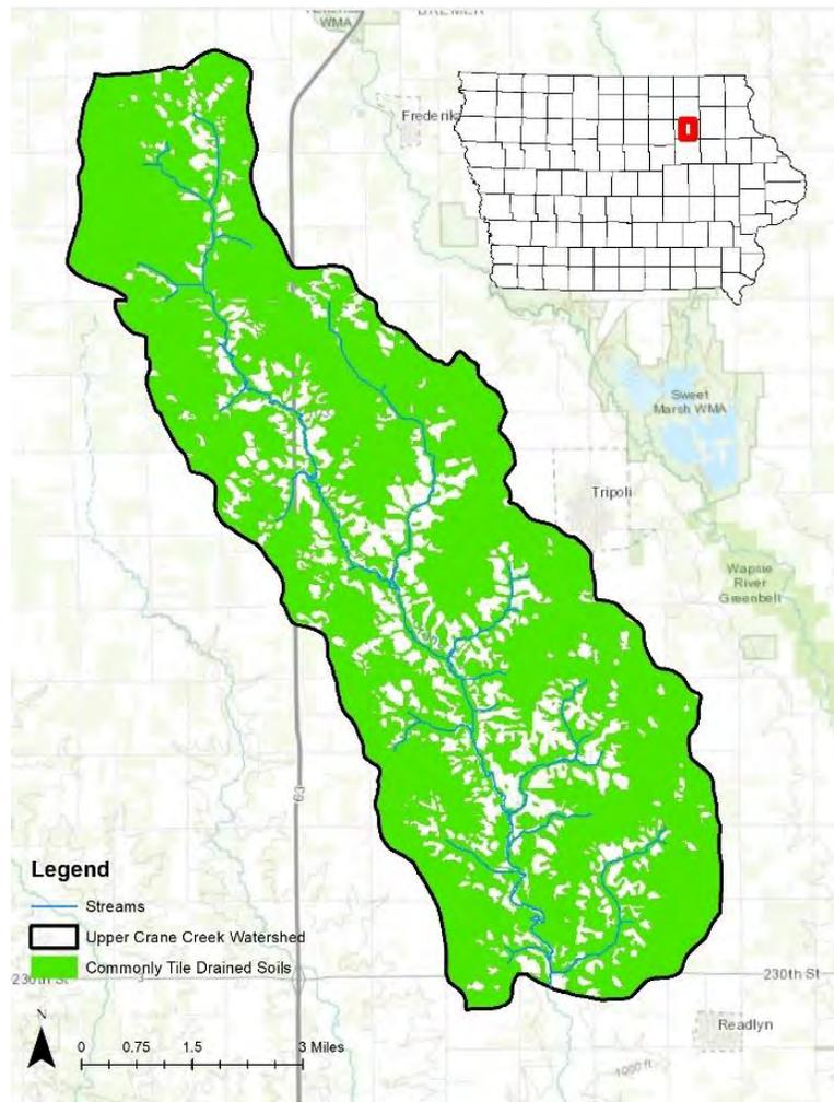
Figure 2.5.3. Areas in the Upper Crane Creek Watershed with likely tile drainage to optimize agricultural production.
