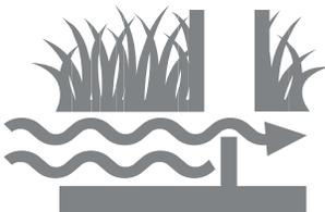
**Drainage Water Management** (4,500 acres) A control structure is used to temporarily raise the water table. This reduces the overall amount of drainage throughout the year. Excess water can be drained before field operations by managing the control structure.
