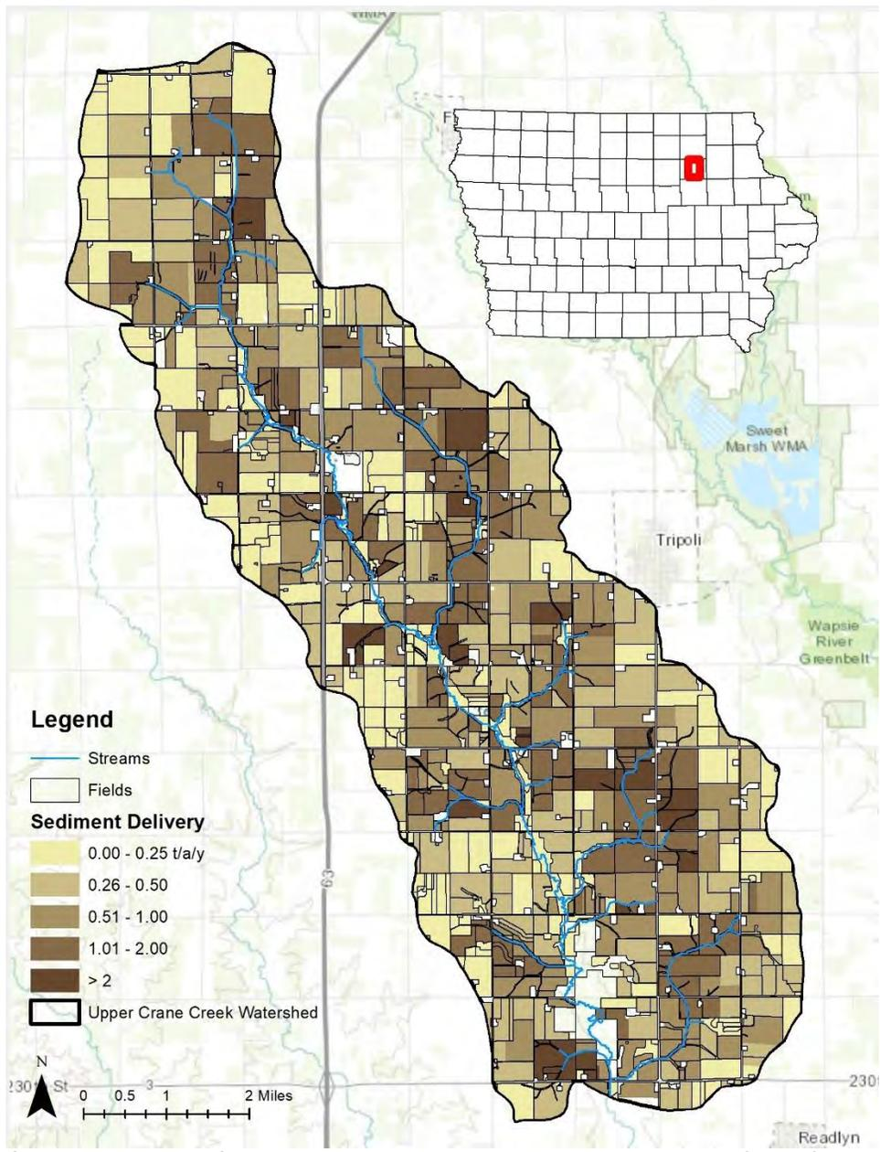
Figure 2.9.3. Estimated rates of upland sediment delivery to streams in the Upper Crane Creek Watershed.
