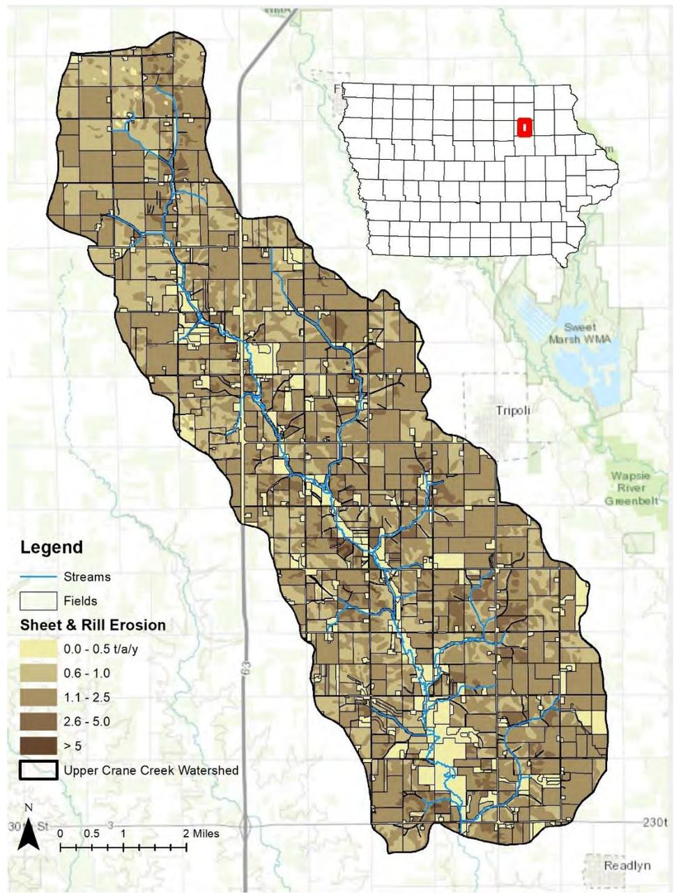
Figure 2.9.1. Estimated sheet and rill erosion rates based on soil types, topography and land use in the Upper Crane Creek Watershed.
